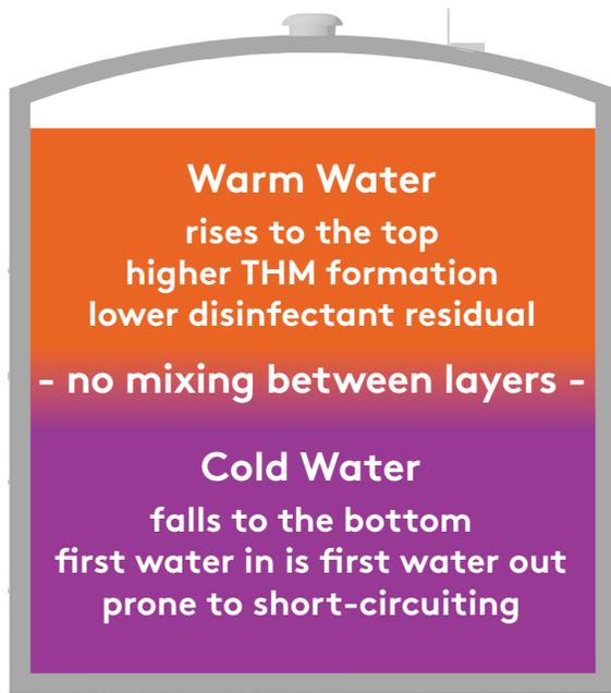
However, a fully and consistently mixed storage system provides a reliable means for true testing of water quality parameters, including temperature and residual disinfectant, from any sample point.
