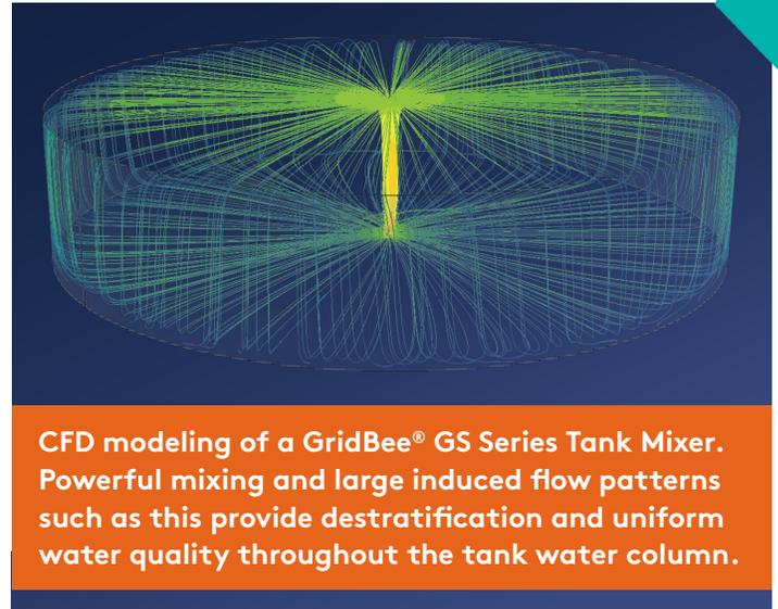
on a regular basis to ensure it meets requirements. Active mixing ensures uniformity in the water column which creates a much higher confidence and trust in water quality testing results. Additionally, both over-chlorination (higher costs) and under-chlorination (higher risk) can be avoided when disinfectant boosting is needed.
