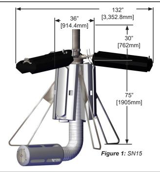
Intake - 20 to 100+ feet (6 to 30+ m) available in 12-inch (30.5 cm) diameter X 20 feet (6 m) sections, thermoplastic rubber, NSF/ANSI 61 approved. Includes low elevation intake that draws water in a horizontal layer within 18 inches (45 cm) of the tank or reservoir floor. Includes intake retrieval chain constructed of 316 stainless steel.
