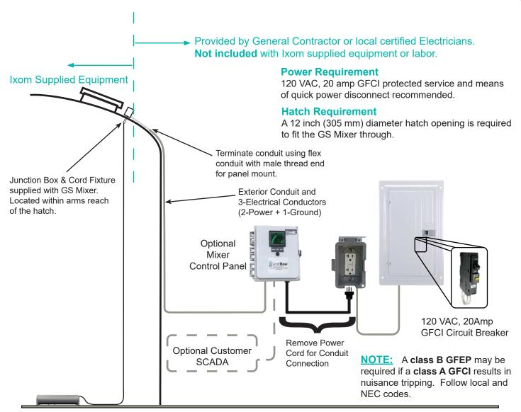
Figure 1: Typical GS Placement
