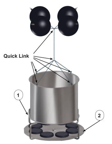
Figure 1: AP Unit Floating Configuration
