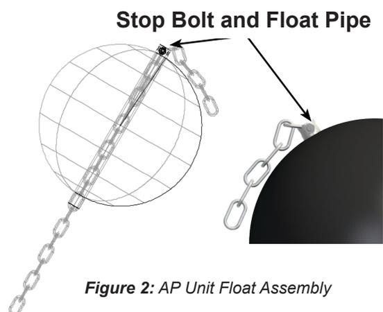
Figure 2: AP Unit Float Assembly
