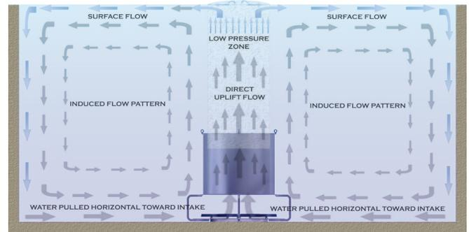
Figure 1: AP Unit Pedestal Configuration Flow Pattern
