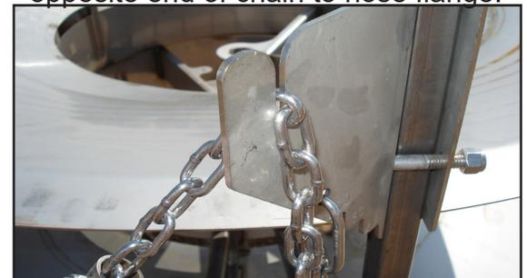
Marker chain slipped into chain bracket slot.
