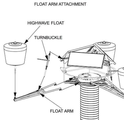
**STEP 1:** Locate the 3 High Wave float arm. Have the M12 x 120mm long bolts and M12 nylok nuts easily accessible near the core unit assembly.
