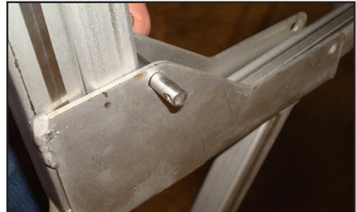
Attaching Leg Extension With a Clevis Pin
