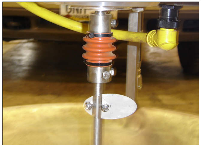
Brushless Motor With Shaft Coupling Attached
