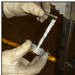
Applying Anti-Seize To The Bolts
