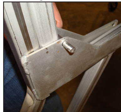
Attaching Leg Extension With a Clevis Pin
