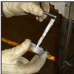
Applying Anti-Seize To The Bolts
