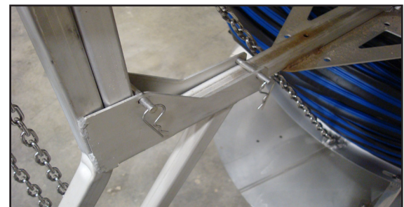
Secured with Hair pins
