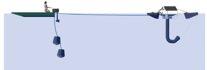
Mooring Blocks Suspended, Ready To Move
