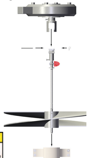
Impeller Assembly Removal Motion
