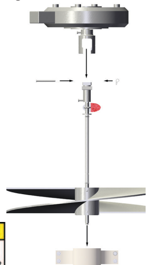
Impeller Assembly Removal Motion
