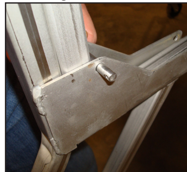
Attaching Leg Extension With a Clevis Pin
