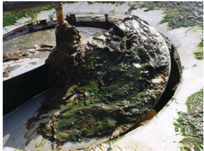
Machine With Buildup On Impeller
