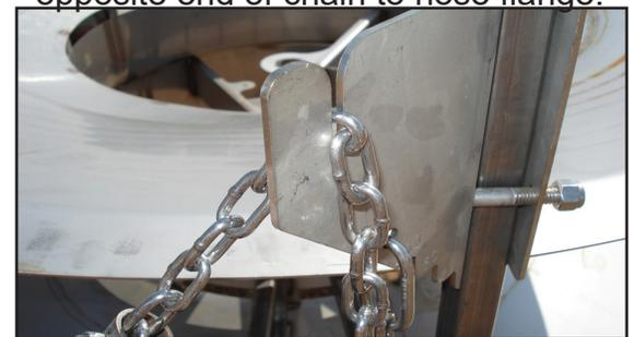
Marker chain slipped into chain bracket slot.
