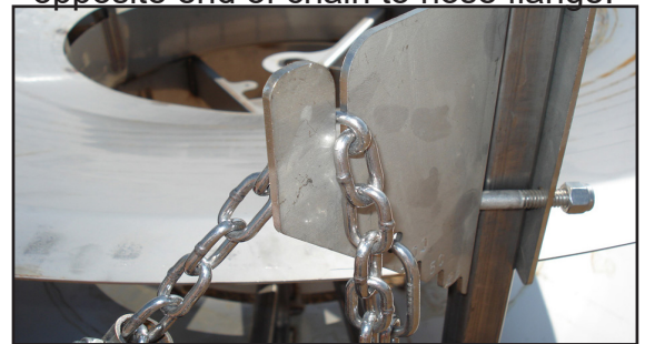
Marker chain slipped into chain bracket slot.
