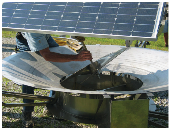
Impeller Removal For Buildup Below Impeller
