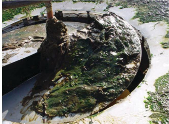
Machine With Buildup On Impeller
