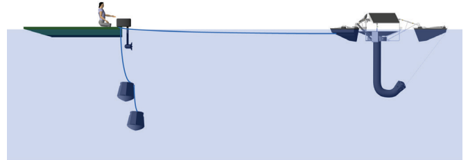
Mooring Blocks Suspended, Ready To Move
