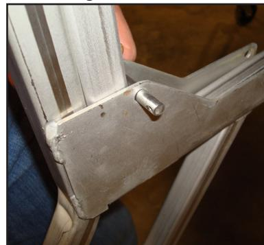
Attaching Leg Extension With a Clevis Pin
