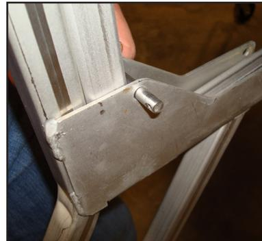
Attaching Leg Extension With a Clevis Pin
