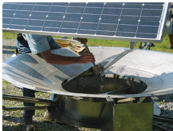
Impeller Removal For Buildup Below Impeller
