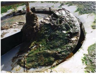
Machine With Buildup On Impeller
