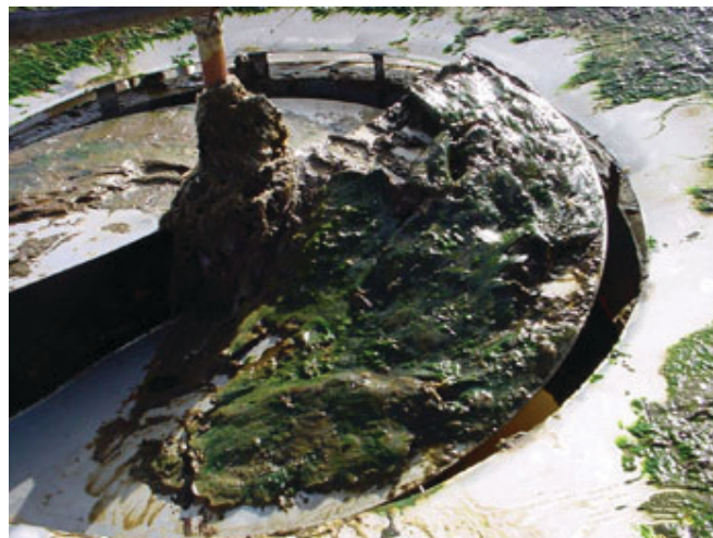
Machine With Buildup On Impeller
