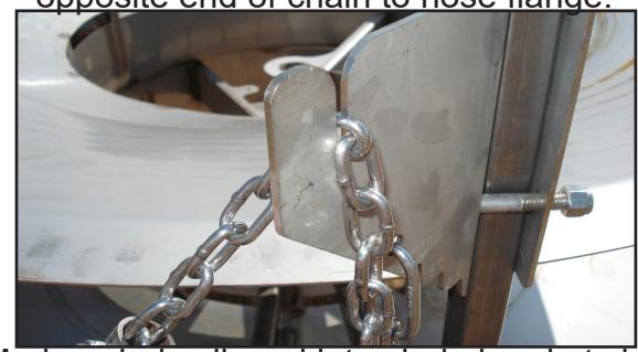
Marker chain slipped into chain bracket slot.
