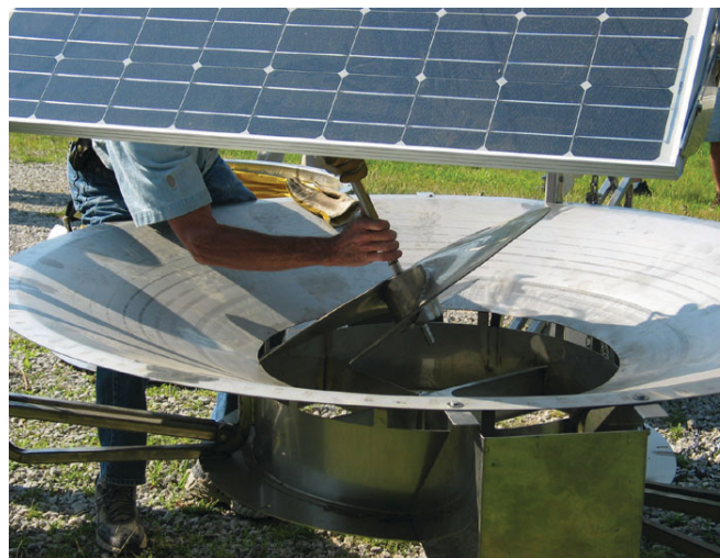
Impeller Removal For Buildup Below Impeller
