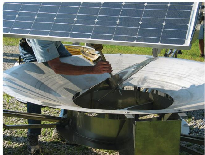
Impeller Removal For Buildup Below Impeller
