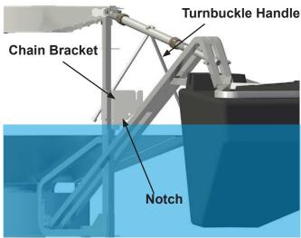
Water Level Even With Notch On Chain Bracket
