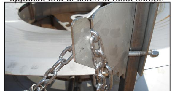
Marker chain slipped into chain bracket slot.
