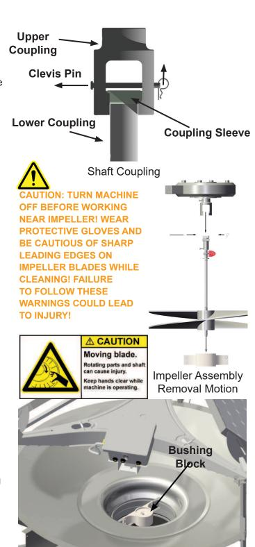
Impeller Assembly Removed
