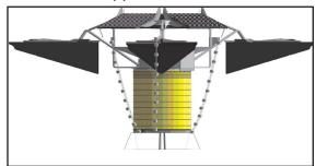
Machine equpped with 3 marker chains.
