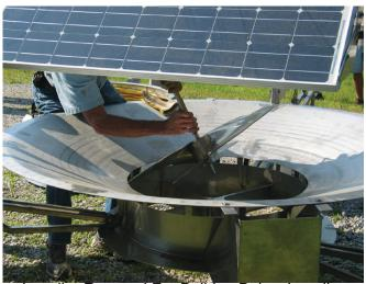
Impeller Removal For Buildup Below Impeller
