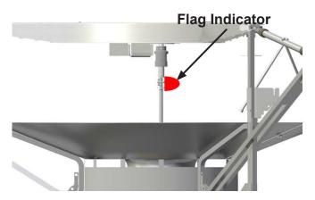
Flag Indicator Section of Impeller Shaft
