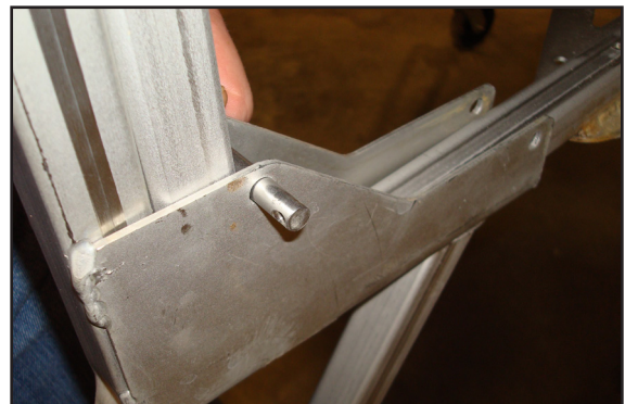
Attaching Leg Extension With a Clevis Pin.
