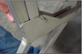
Sliding Leg Extension Around Bottom Leg Of Machine Core Unit
