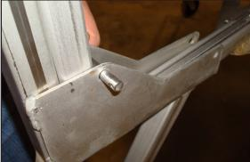
Attaching Leg Extension With a Clevis Pin.
