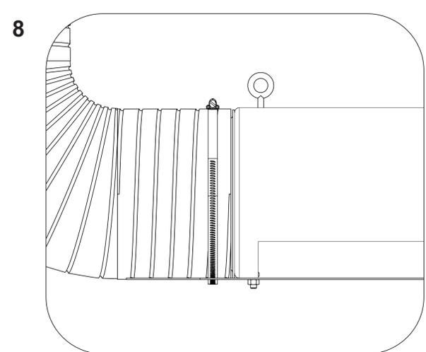
**STEP 1:** Locate one end of the hose section and place hose clamp over the end. Be sure that hose and clamp are installed above the metal rib of the flange and then tighten hose clamp as tight as possible to firmly secure hose. **(See Figure 5)**
