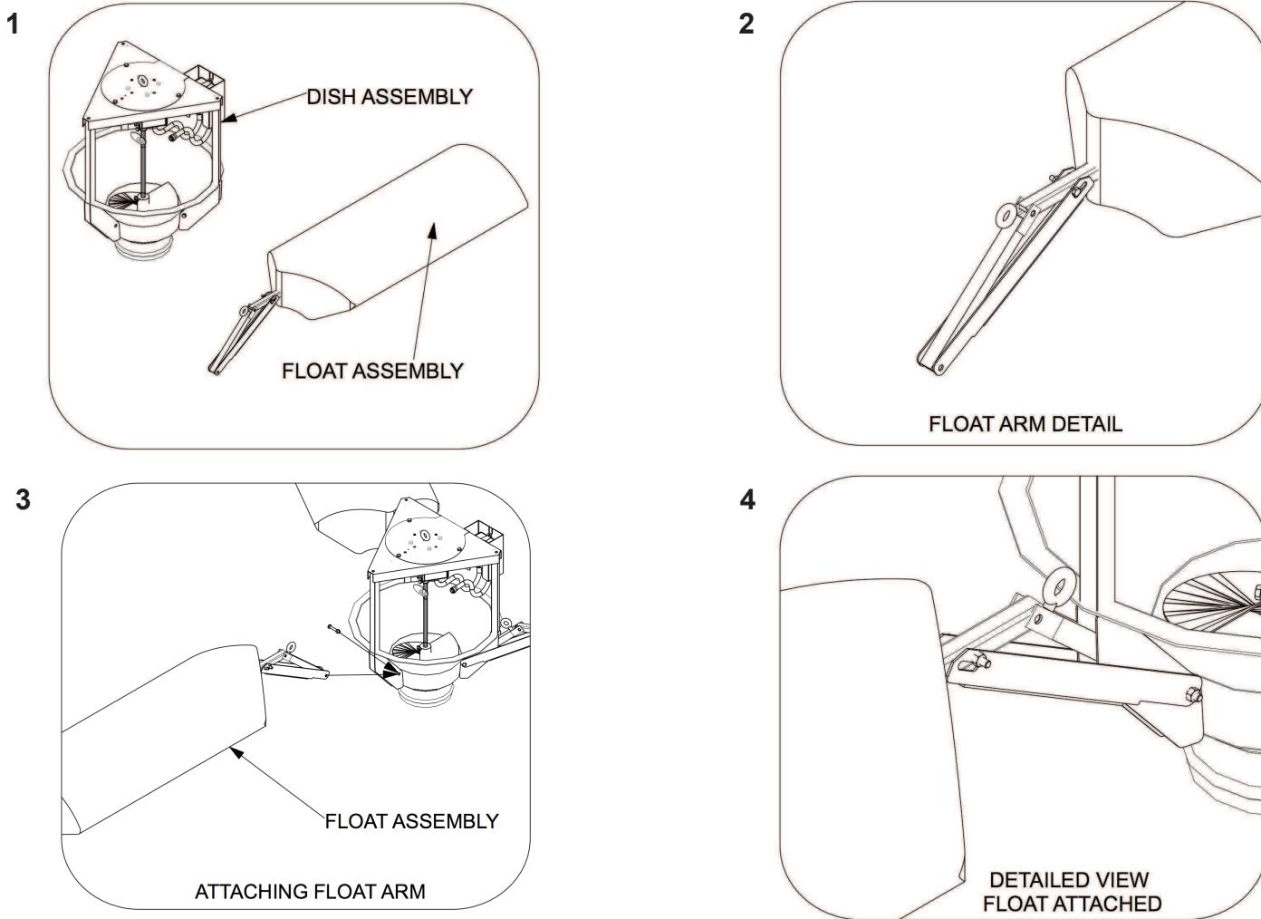
**STEP 1:** Locate the Dish Assembly and Float Arm Assembly. **(See Figure 1 & 2)**
