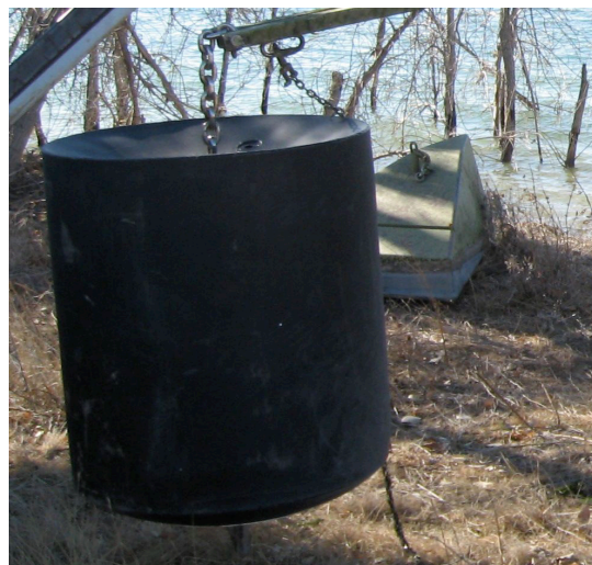
Float upside down chain end toward float arm
