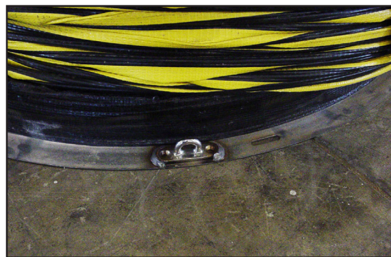
Weld link on hose flange connecting opposite end of chain to hose flange.
