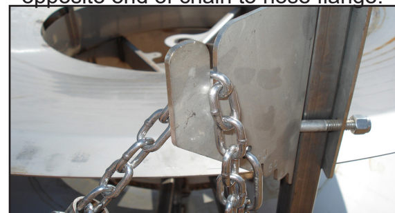
Marker chain slipped into chain bracket slot.
