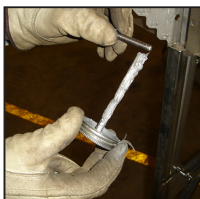
Applying Anti-Seize To The Bolts
