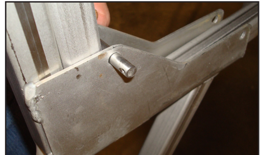
Attaching Leg Extension With a Clevis Pin
