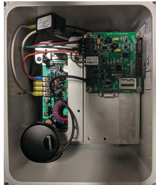
*Figure 2: SB A-Series Control Panel, Internal*
