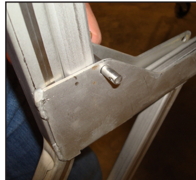
Attaching Leg Extension With a Clevis Pin
