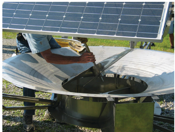
Impeller Removal For Buildup Below Impeller
