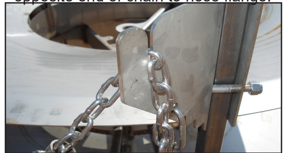
Marker chain slipped into chain bracket slot.
