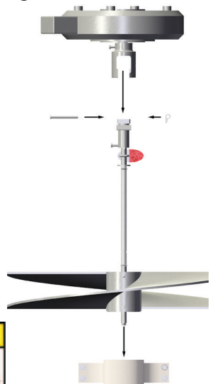
Impeller Assembly Removal Motion
