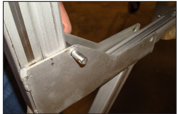
Attaching Leg Extension With a Clevis Pin.
