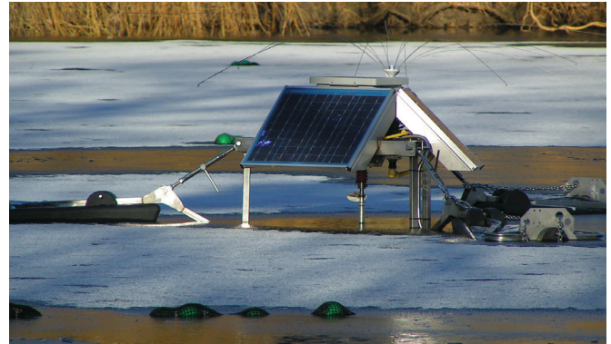
SolarBee In A Lake That Is Partially Frozen
