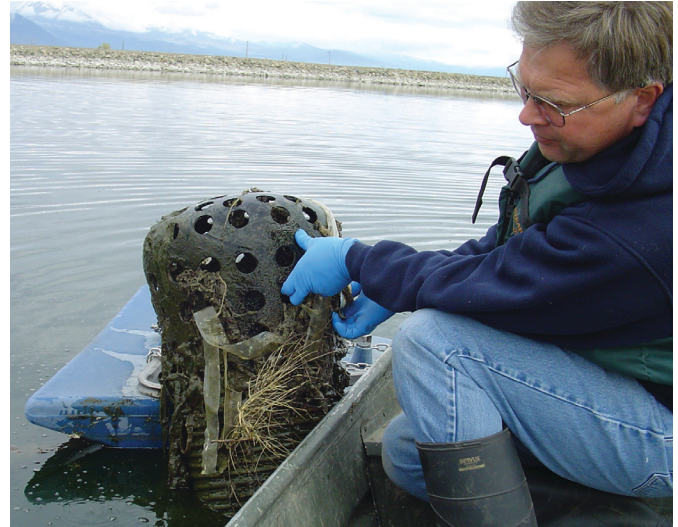
Partially Plugged Strainer
