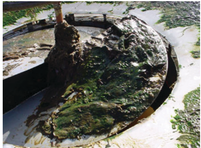
Machine With Buildup On Impeller
