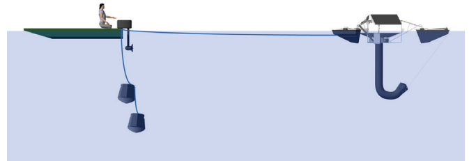
Mooring Blocks Suspended, Ready To Move
