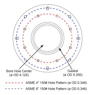
Figure 3: Flange Bolt Pattern Outside Tank
