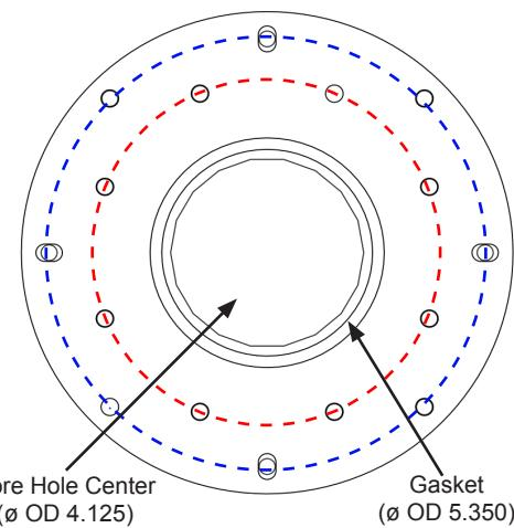
Figure 3: Flange Bolt Pattern Outside Tank
