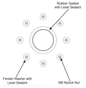
Figure 4: Bolt View Inside Tank
