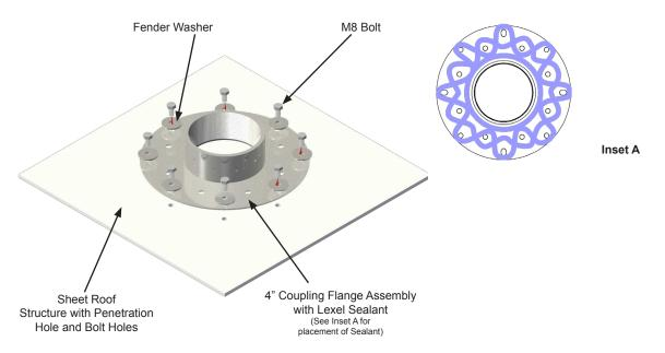
Figure 1: Outside Tank Bolt Installation
