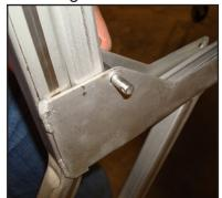
Attaching Leg Extension With a Clevis Pin
