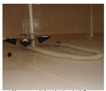
Hose properly layed out on tank floor.
