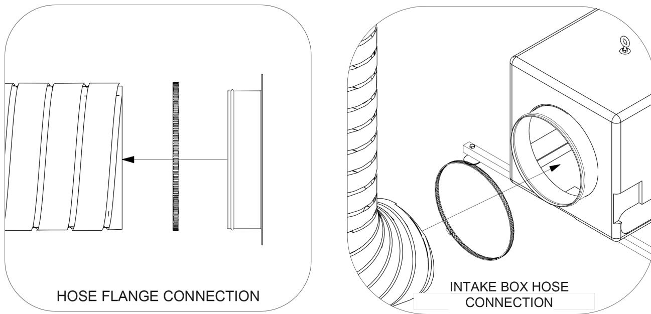
**STEP 1:** Locate one end of the hose section and place hose clamp over the end, and insert a hose flange. Repeat on opposite end of the hose section. Be sure that hose and clamp are installed above the metal rib of the flange and then tighten hose clamp as tight as possible to firmly secure hose.
