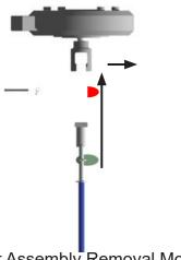
Impeller Assembly Removal Motion
