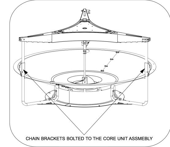
CHAIN BRACKETS BOLTED TO THE CORE UNIT ASSMEBLY
