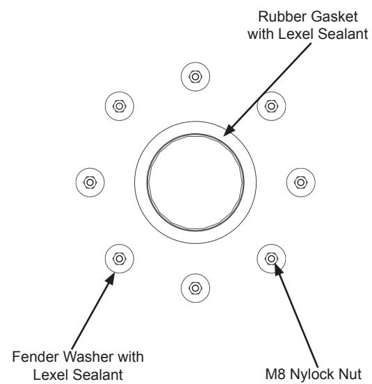
Figure 4: Bolt View Inside Tank
