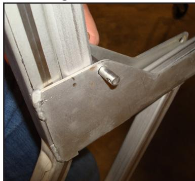
Attaching Leg Extension With a Clevis Pin
