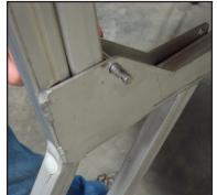
Sliding Leg Extension Around Bottom Leg Of Core Unit
