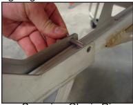
Securing Clevis Pins
