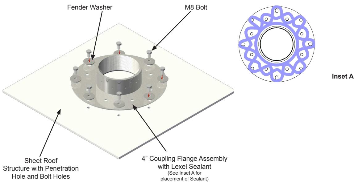
**Figure 1:** Outside Tank Bolt Installation
