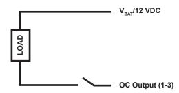
Figure 1: OC Output Wiring
