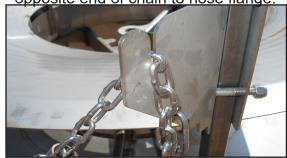
Marker chain slipped into chain bracket slot.
