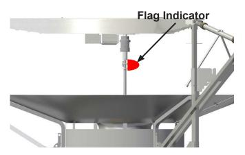
Flag Indicator Section of Impeller Shaft
