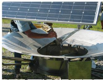
Impeller Removal For Buildup Below Impeller
