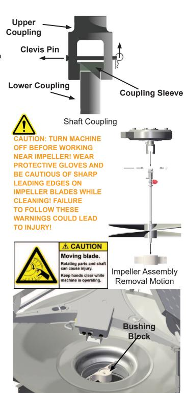
Impeller Assembly Removed
