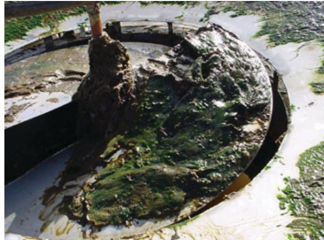
Machine With Buildup On Impeller
