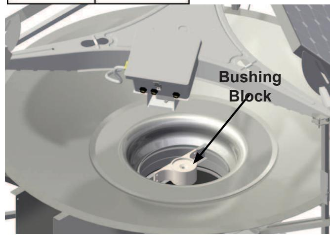
Impeller Assembly Removed
