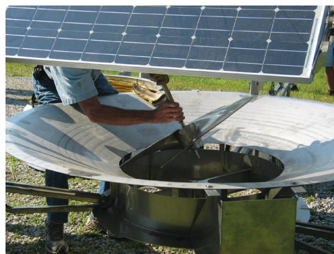
Impeller Removal For Buildup Below Impeller
