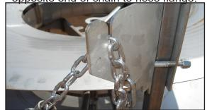
Marker chain slipped into chain bracket slot.
