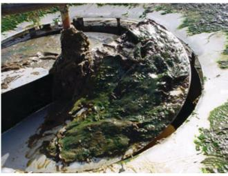
Machine With Buildup On Impeller
