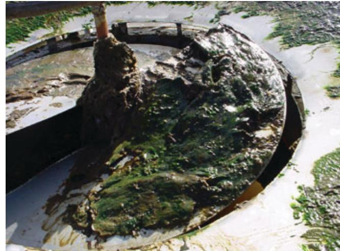
Machine With Buildup On Impeller
