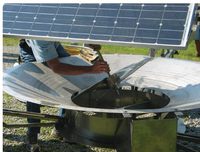
Impeller Removal For Buildup Below Impeller
