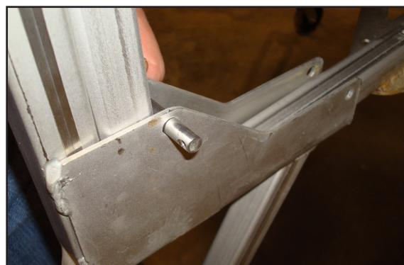
Attaching Leg Extension With a Clevis Pin.
