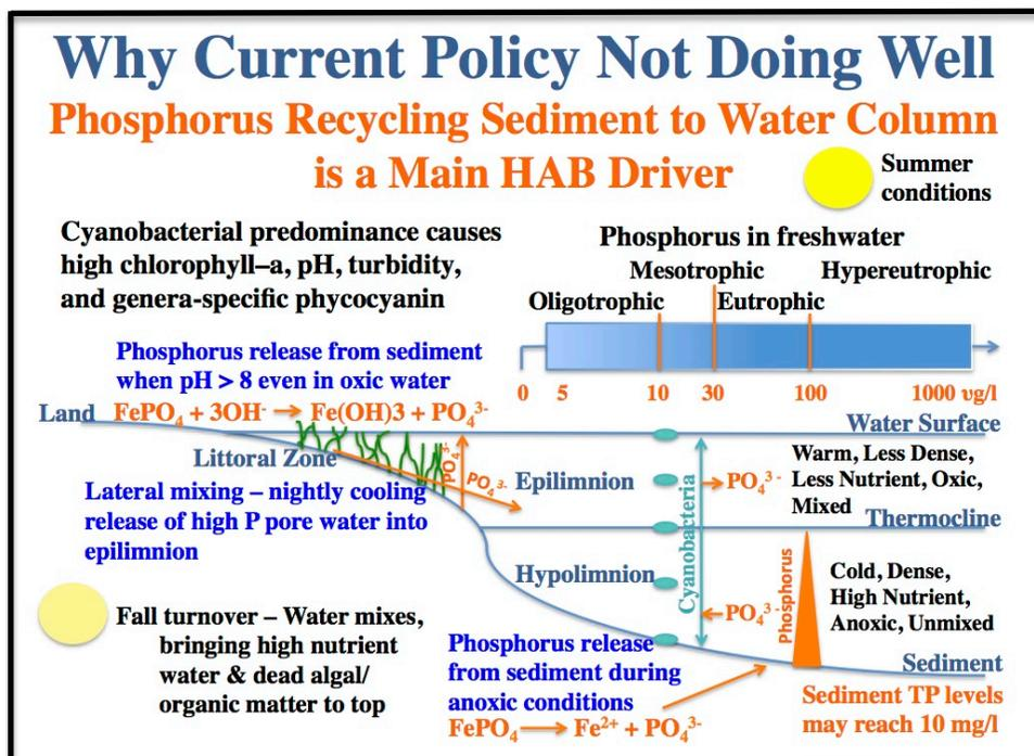
Figure 3. Phosphorus moves from sediment into the water column during anoxic conditions. Second, phosphate releases from iron when pH > 8 even during oxic conditions. Third, when air above the water surface is cooler than the surface water, thin surface layers cool, become denser, and fall through the water column while deeper, warmer layers rise. This process causes both lateral mixing and “fall turnover.”
