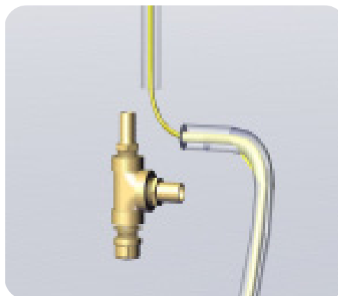
Figure 10: Step 6, 7 & 8 Attach Exterior Hose to Drain Assembly
