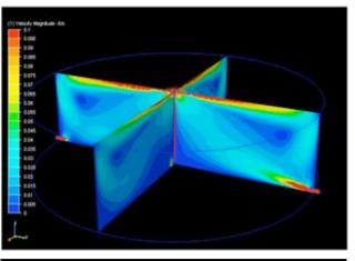
**Figure 2.** Computational Fluid Dynamics Modeling comparable to that shown in Figure 1 except that a SB1250PW is circulating the 2 MG of water. Continual mixing eliminates thermal stratification and prevents ice buildup.
