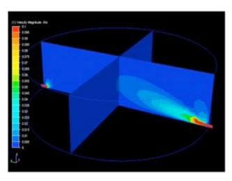
**Figure 1.** Computational Fluid Dynamics Modeling of a 2 MG tank with separate influent and effluent pipes indicates that most of the water is stagnant (blue) even during strong inflow (right, red) and moderate outflow (left, red).
