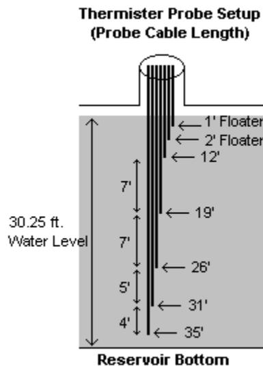
**Figure 5: Example of Thermistor Setup**
