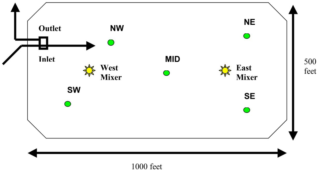
Figure 2: Diagram of Sunset Reservoir South with Sample Station Locations and Recommended Placement of Mixers by Solarbee.
