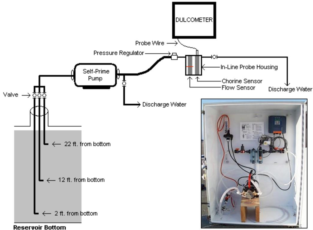
Figure 3: Example of Monitoring Station and Pump Setup Located on Reservoir Roof
