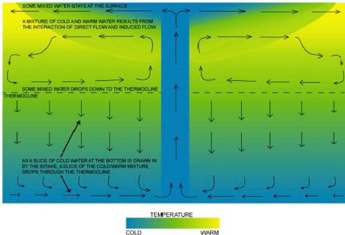
Figure 12: Diagram of Solarbee Flow Pattern During Stratified Conditions (Solarbee, 2003)
