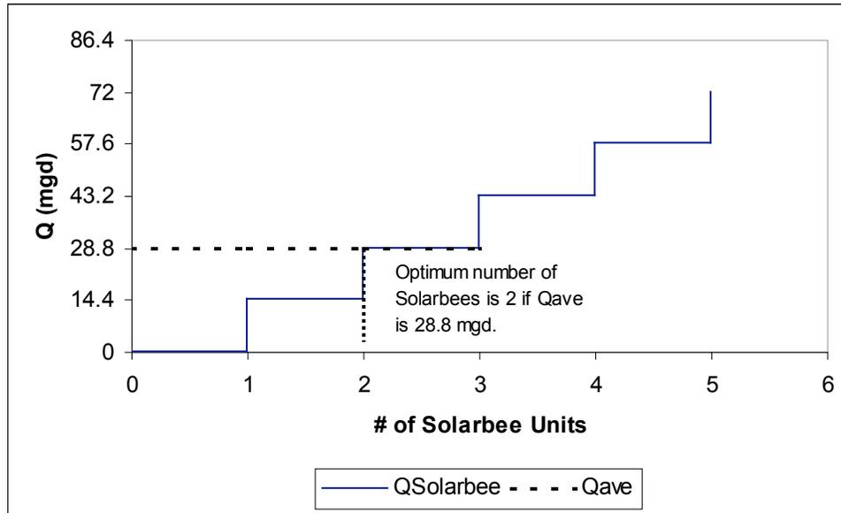
Figure 13: Estimated Number of Solarbee Units Required for In-Service Conditions
