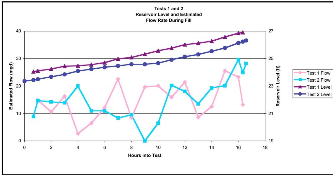
Figure 6: Graph of Reservoir Levels and Estimated Flow Rates for Tests 1 and 2<sup>13</sup>
