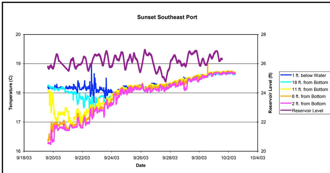
**Figure 4: Example of In-Service Stratified Conditions Returning to Mixed Conditions between Summer and Fall—No Mixers.**
