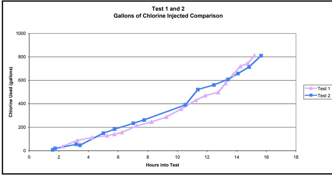
Figure 7: Comparison of Chlorine Gallons Injected – Tests 1 and 2
