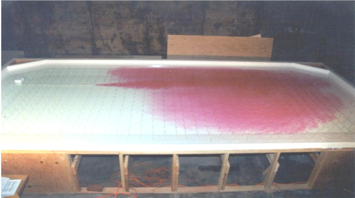
**Figure 8: Example of Test 1 and 2 Flow Pattern – Taken from “Physical Modeling Studies of Sunset South” (Hydroconsult Engineers, 2001)**
