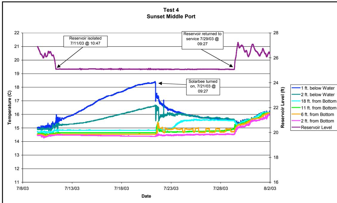
Figure 11: Example of Test 4 Thermistor Data – Decrease of Stratification by Solarbee
