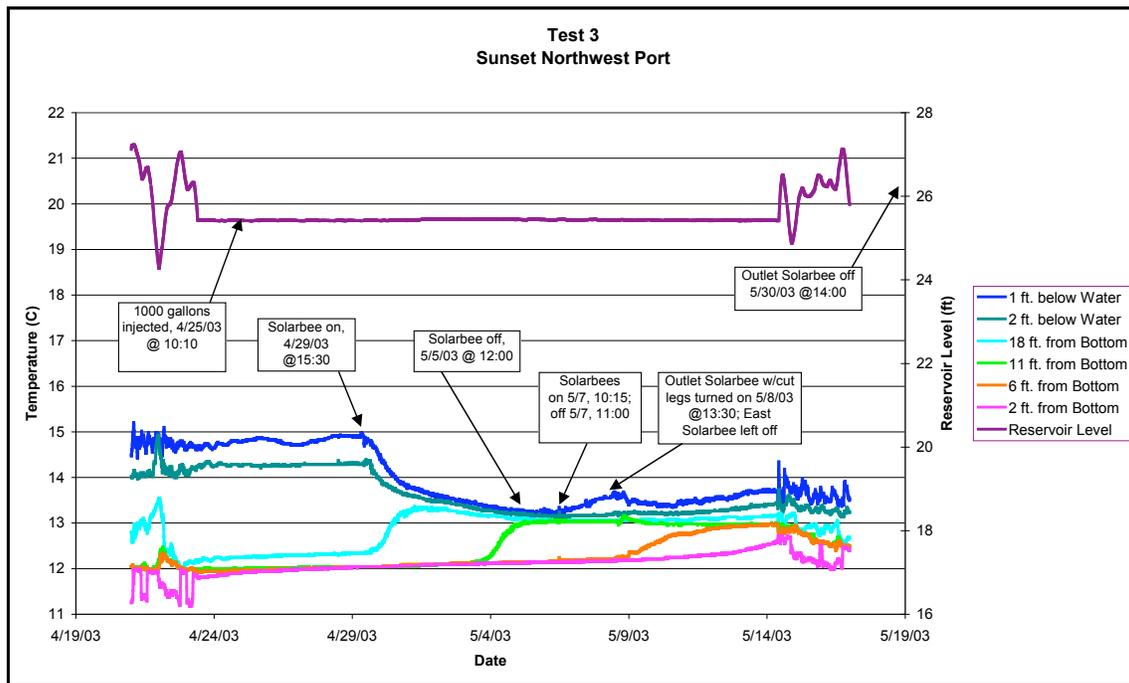
**Figure 10: Example of Test 3 Thermistor Data – Decrease of Stratification by Solarbee**
