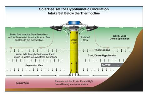
To access educational lake videos and information, please visit us at www.ixomwatercare.com **Hypolimnetic Circulation-** The intake is set deep in the reservoir below the thermocline to continuously bring up and expose bottom waters to the oxygen-rich epilimnion and atmosphere.
