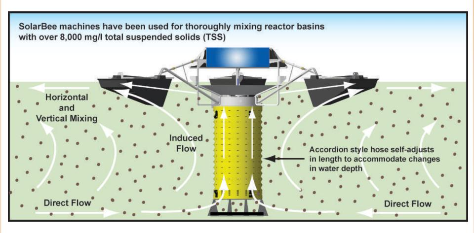
Water and suspended solids (TSS) from across the bottom of the basin enter the hose just above the floor, travel up the hose, and are then spread across the surface
