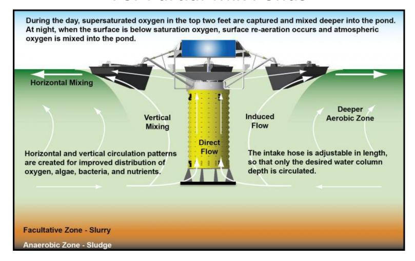
With the intake plate set above the slurry and sludge at the bottom of the pond, the water, bacteria, and oxygen can be thoroughly mixed without disturbing the bottom
